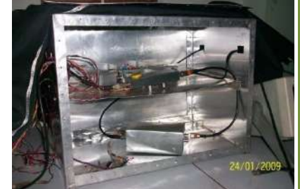
Various instruments are fabricated at ICSP laboratory to be flown to the Stratosphere by 100ft long Hydrogen filled balloons at a height of ~ 42 km. ICSP also made climate chambers to test payloads before launching.
